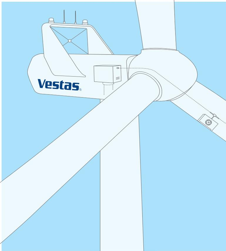
The turbine controller monitors power performance and takes input from climatic sensors and turbine operating parameters.
